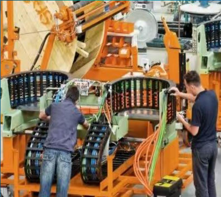
**Drag Chain Harness and flexible-bending cable for industrial robots**
