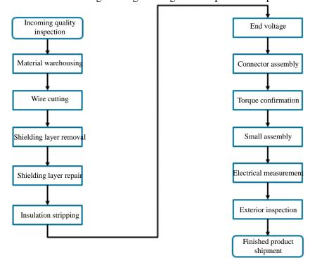
5. Computer peripheral products and parts turnkey processing flow
